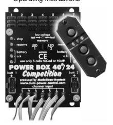
Featuring seven servo-pulse amplifiers plus two independent voltage-controllers
