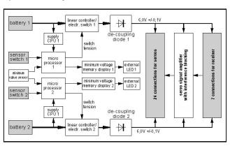
When long servo leads are used there is a danger of RF interference signals reaching the receiver by that route, but the integral servo signal amplifiers also effectively prevent this by blocking the interference. For this reason ferrite rings are not required for de-coupling the servo cables when this backer is used.
